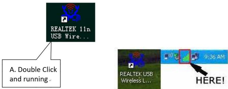
7. After finishing driver installation, click adapter utility from your taskbar or programs folder. Click "**available networks**", select the wireless access point you would like to connect and press "**Add to Profile**" button.
